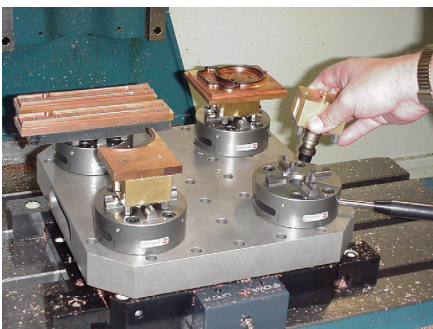
ITS chuck: Also suitable for installation in special fixtures.
